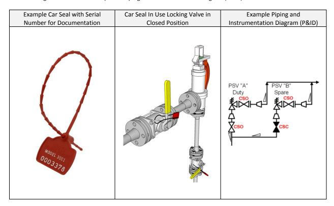
Car seals are generally used to seal a rail car, truck, cargo container or other openings to prevent/indicate tampering are also used in industry processes. A car seal is typically placed on a valve but it can be placed on any type of physical equipment to prevent unauthorized operation.
